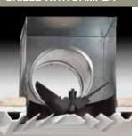
Model GRD grille/damper combination for low clearance side or top entry applications. Same construction as MV diffusers but with no boot. Standard 8" size only. Available in all five grille styles.
