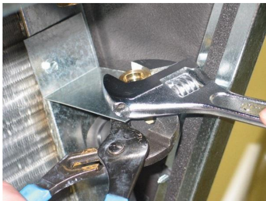
Figure 23. Remove Nut
