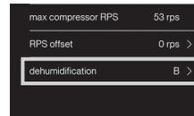
15. Select one of the settings according to your demand at this display. “off” means no special dehumidification profile setting. “A” has the less dehumidification performance than the default setting “B”, while “C” has the maximum performance.
