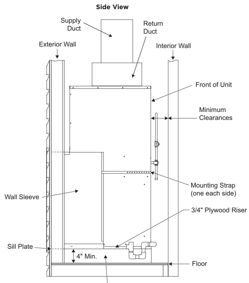
Platform (field supplied) - Unit must be supported by platform, which must be level with sill plate of opening in exterior wall.
