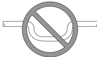
Fig. 21 - Insufficient Condensate Trap
