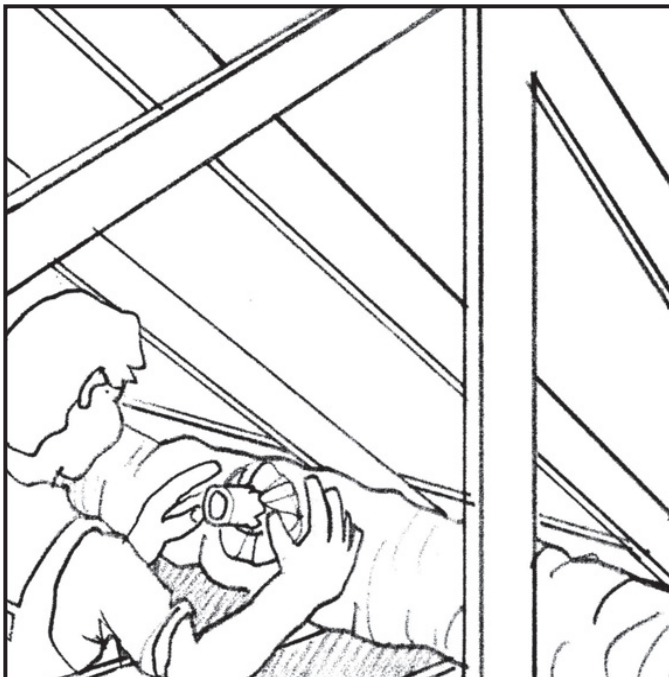
Fig. DUC-11 - BTO with insulation sleeve
