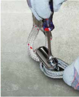
Replace and tighten pin
