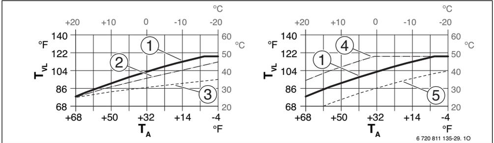
Fig. 13 Settings for heating curve with **Low Temp.** heating
