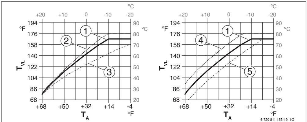
Fig. 14 Settings for heating curve with **High Temp** heating
