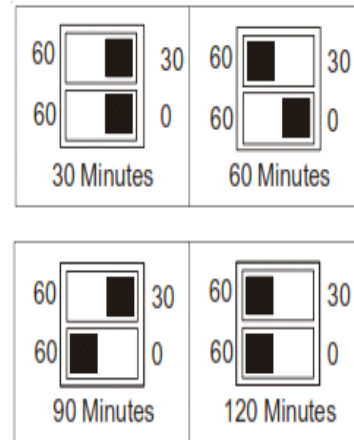
Dipswitch Settings for Selection of Defrost Time
