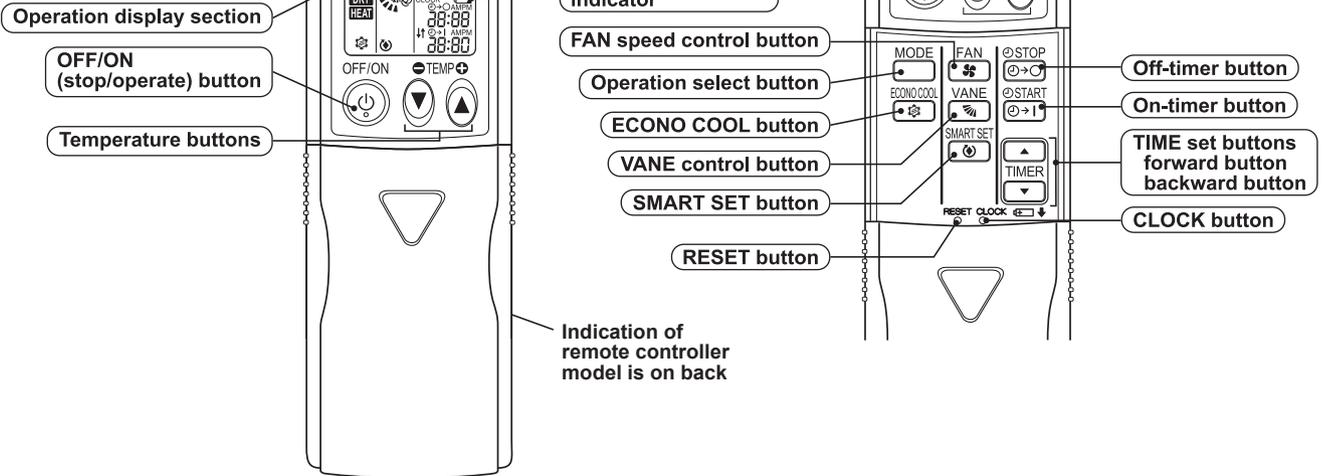
**NOTE:** Last setting will be stored after the unit is turned OFF with the remote controller. Indoor unit receives the signal of the remote controller with beeps.
