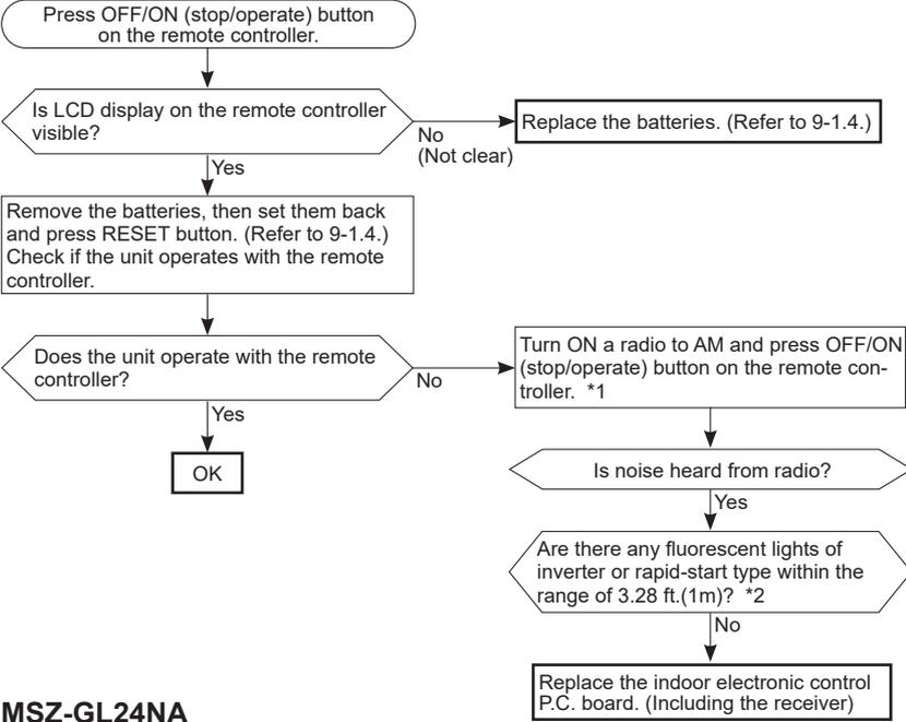
\*1 Look at the image of the signal transmitting section of the remote controller through the monitor of a digital camera or a camera phone. It is normal if the LED of the signal transmitting section lights up when the OFF/ON (stop/operate) button on the remote controller is pressed. However, it may be difficult to see the illuminated LED of the signal transmitting section with a smartphone camera.
