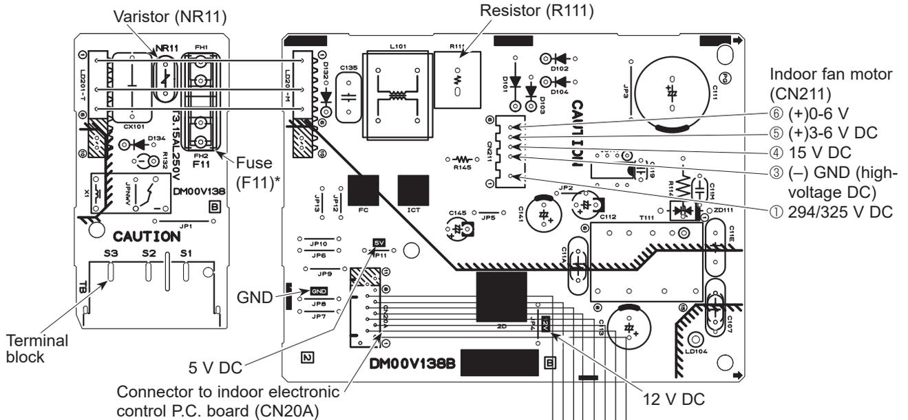
\* Please replace the fuse after removing the indoor terminal P.C. board from the electrical box.
