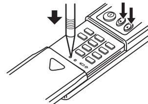
Press RESET button gently using a fine-tipped object.
