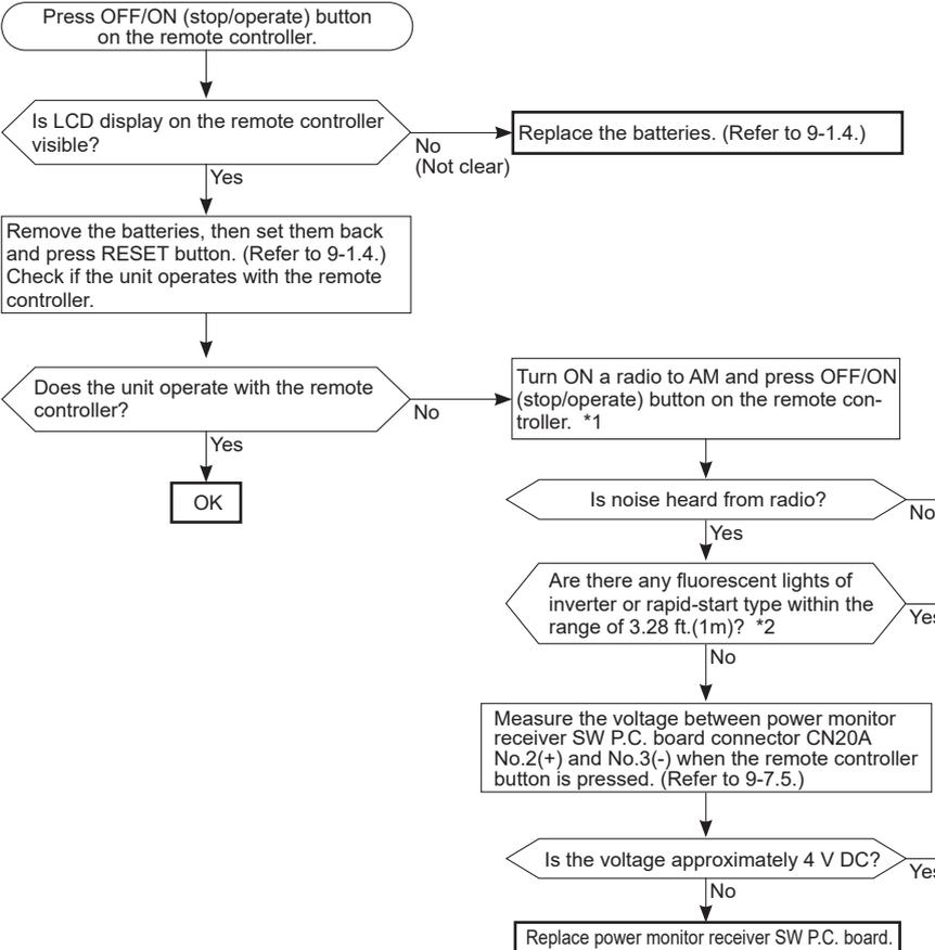
\*1 Look at the image of the signal transmitting section of the remote controller through the monitor of a digital camera or a camera phone. It is normal if the LED of the signal transmitting section lights up when the OFF/ON (stop/operate) button on the remote controller is pressed. However, it may be difficult to see the illuminated LED of the signal transmitting section with a smartphone camera.
