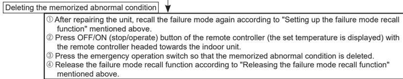
**NOTE:** 1. Make sure to release the failure mode recall function after it is set up, otherwise the unit cannot operate properly.
