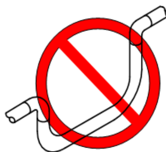
FIGURE 3. - Insufficient Condensate Trap
