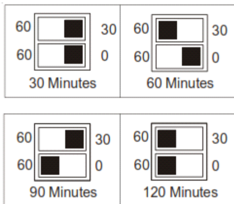
Dipswitch Settings for Selection of Defrost Time
