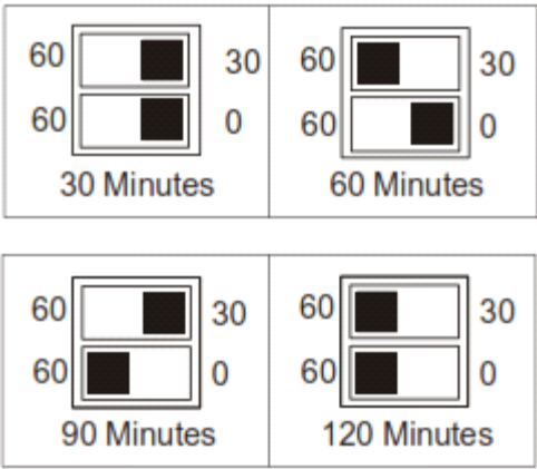
Dipswitch Settings for Selection of Defrost Time
