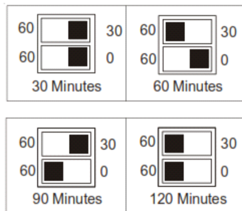
Dipswitch Settings for Selection of Defrost Time
