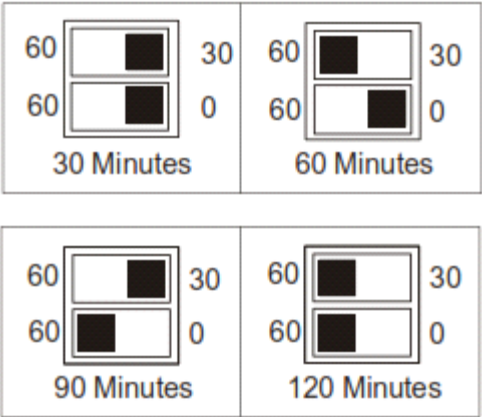
Dipswitch Settings for Selection of Defrost Time
