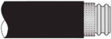
Proper FlashShield End Prep
