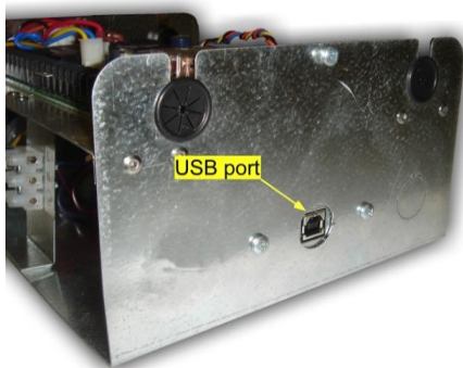
Figure 19. Location of USB (computer) port
