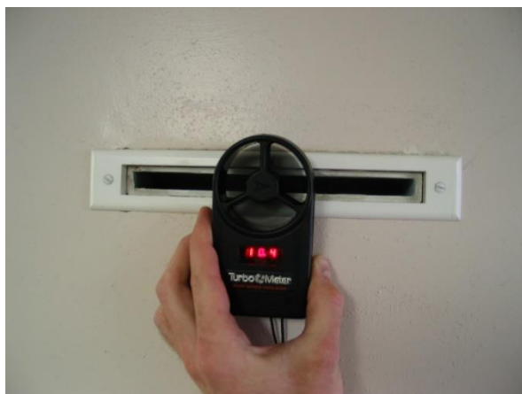
Figure 8. TurboMeter Placement for Slotted Outlets
