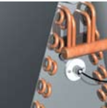
Custom lamp flange allows lamp to be installed directly in A-coil delta plate for optimal UV exposure.
