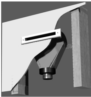
Figure 2. Typical Wall Installation, 90° Outlet
