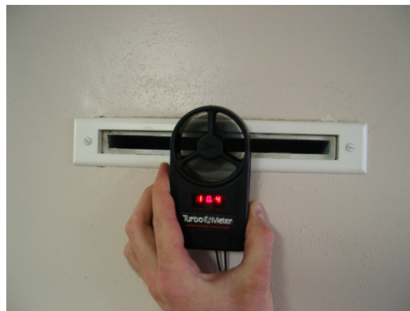
Figure 7. TurboMeter Placement for Slotted Outlets
