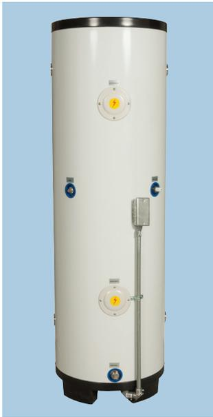
As a hydraulic separator, BT's separate the hydronic from the energy source loop (heat pump / boiler) from the hydronic flow in the distribution system (air handlers / emitters). Hydraulic separation is used primarily in systems where flow rates from the source to the distribution vary or with applications utilizing variable speed pumps. The heating or cooling source can be hydraulically decoupled from the distribution system.
