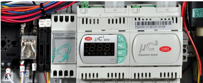
Intelligent factory configured control platform, with state-of-the-art self diagnostic microprocessor allow staging of compressors for seamless operation. Amp draw starts low and stays low with no spike at start-up and use a smaller breaker than other heat pump units for even more efficiency benefits.
