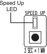
The Speed Up button can be used to put the internal panel time delays in speed up mode. When the button is pushed, the Speed Up LED will blink. Pushing the button again will reset the time delays and the LED will turn off or will automatically reset in 10 minutes.
