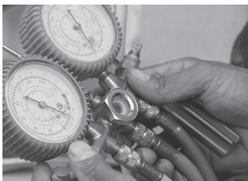
5) With manifold closed, wait one minute for charging hose and Acid Away PRO injector to equalize to suction pressure.
