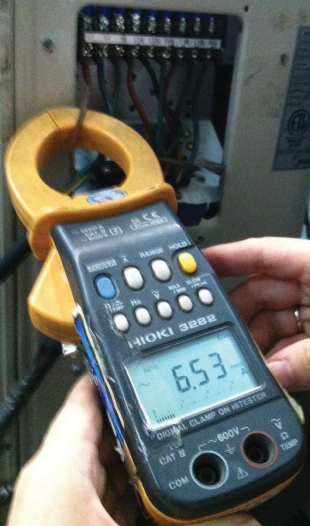
Fig. 66 — Test the voltage
