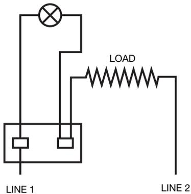
PILOT LIGHT (OPTIONAL) IS OFF WHEN THERMOSTAT SWITCH IS OFF
