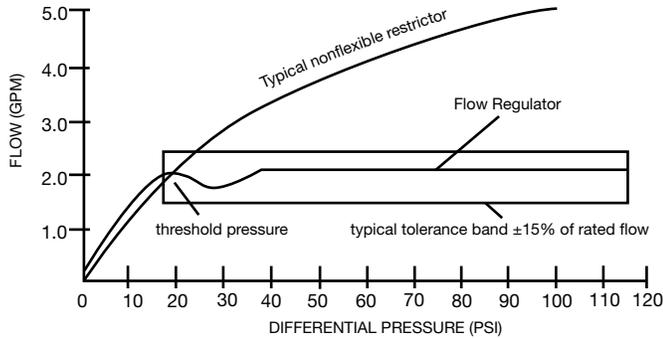
1. Calculated flow through 1/8" diameter orifice
