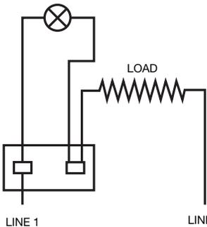
PILOT LIGHT (OPTIONAL) IS OFF WHEN THERMOSTAT SWITCH IS OFF
