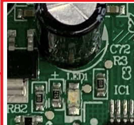
LED1: Drive failure indicator
