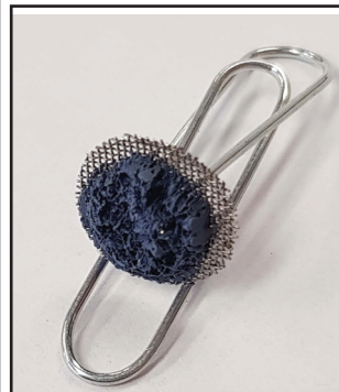
[Fig. 3] - Clogged Filter Screen
