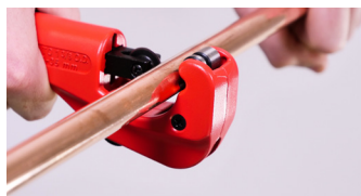
1. Cut the tube to length
