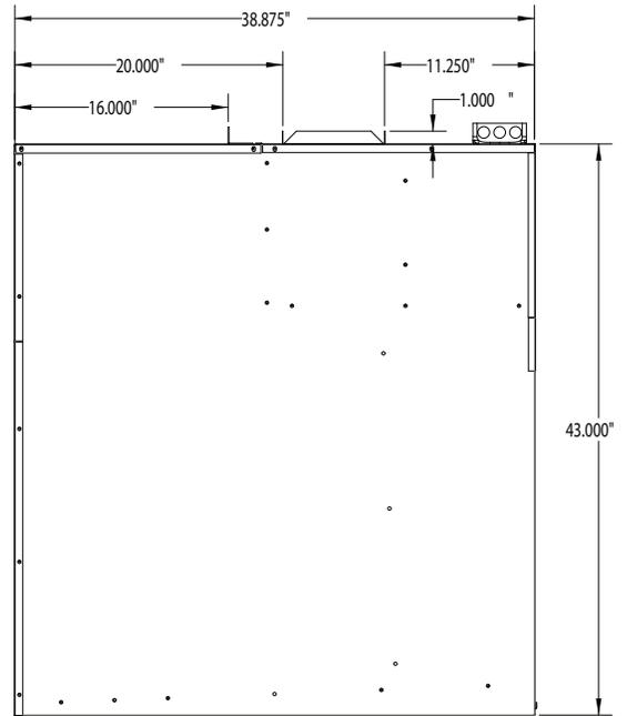
NOTE: Unit must be mounted a minimum of 8 inches above finished floor.
