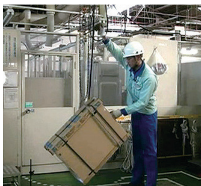
Drop/strength testing
