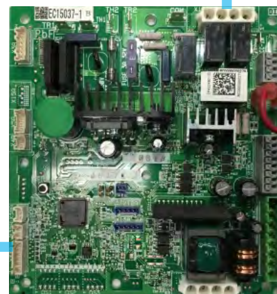
Fig. 8. FXTQ_TA Indoor Unit PCB
