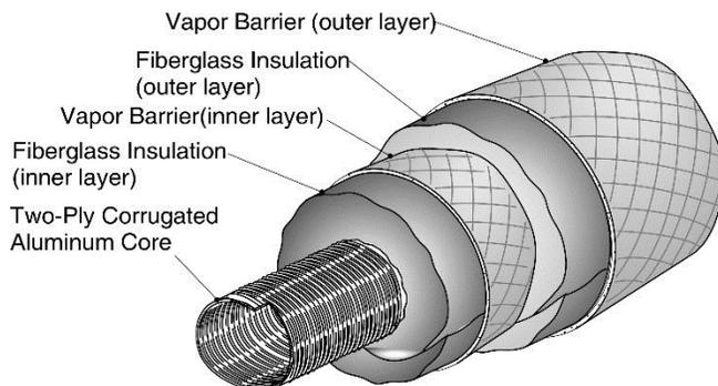
**Figure 3. Typical tubing construction with double vapor barrier**
