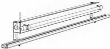
Fig. 4 Strut mount installation with unit bolted to the strut on the short side of the bracket.
