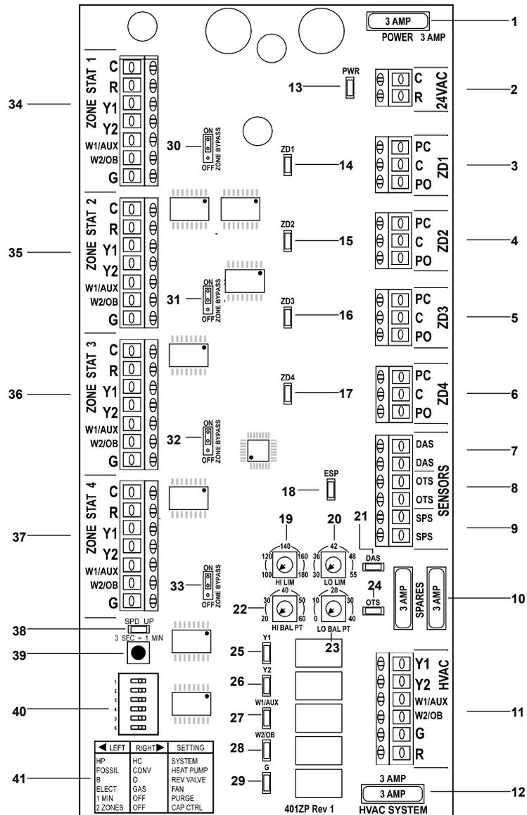
1. 3 AMP FUSE PROTECTS PRINTED CIRCUIT BOARD
