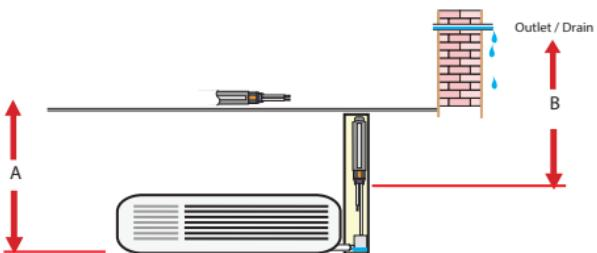
Leave sufficient space around the pump unit to allow for cooling. Ensure that the pump is not more than A above the condensate outlet, and not more than B below the desired drainage point for the pump outlet. The pump can be mounted in any orientation but must be kept DRY. (See table above for A & B). Connect the discharge tube of the pump to a suitable drainage system. Secure with cable ties where necessary. A stepped adaptor is supplied to convert various tube diameters.
