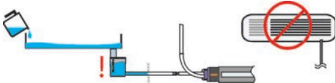
To ensure that the alarm connection is working, restrict the outlet of the reservoir/DrainStik® hose and fill with water up to the high level sensor. The pump will turn on initially, then after a short delay the alarm relay will switch, detected using a multimeter or observing the shut down of the AC unit. Allow the water to exit the reservoir; the water should then be pumped away, and AC operation will restart.
