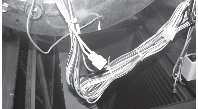
Figure 9: Install 2-Pin Jumper Plug
