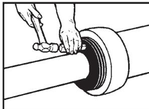
Insert Donut and spigot assembly into the opening. Drive Donut with hammer and wedge until fully seated.
