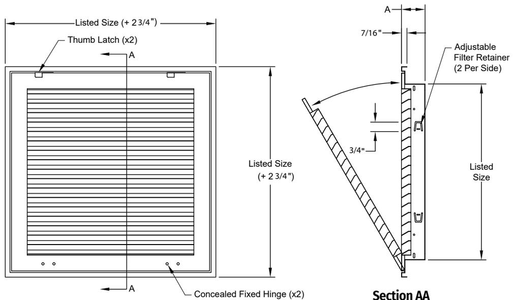
Note: This submittal is meant to demonstrate the general dimensions of this product. The illustrations are not meant to detail every aspect of the product. Drawings are not to scale.
