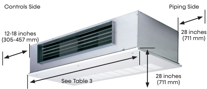
Figure 7: CBY Unit Clearance and Service Access
