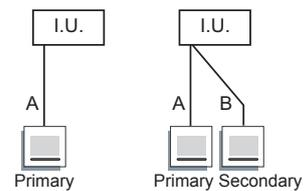
A, B : Remote controller cable. (Refer to 3.3. Electrical requirement.)
