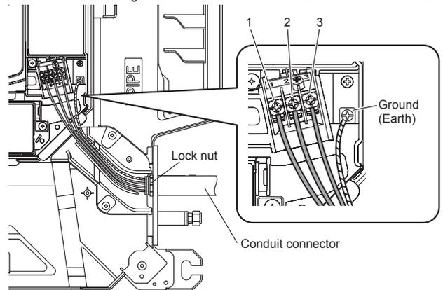
(3) After wiring is complete, secure the cables with the cable clamps.
