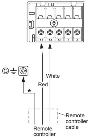
\* : Ground (Earth) the remote controller if it has a ground (earth) wire.
