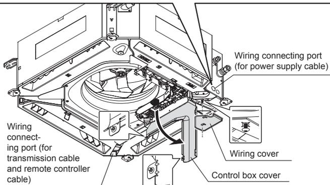
(2) Thread each cable through the holes or indents of the cabinet and connect the wires.
