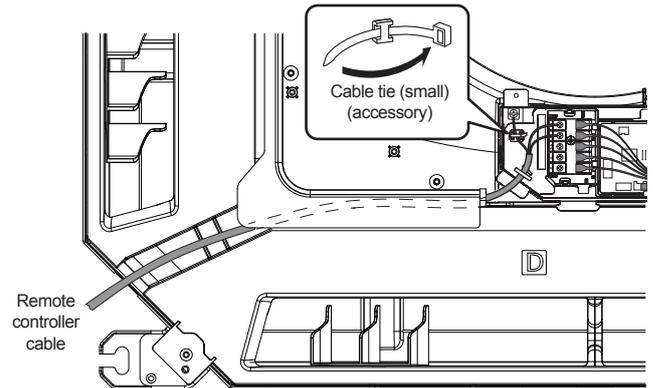
(4) Replace the Control box cover and Wiring cover. Securely tighten the screws.
