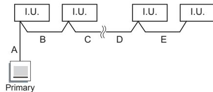
A, B, C, D, E : Remote controller cable. (Refer to 3.3. Electrical requirement.)
