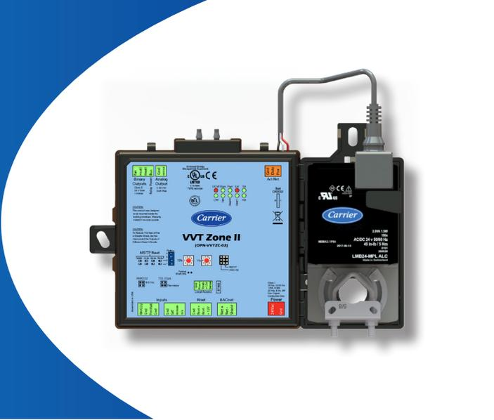
The VVT rectangular zone damper with VVT Zone controller is a component of Carrier's i-Vu Building Automation System. It provides accurate and precise airflow for VVT applications. The factory-integrated VVT Zone controller maintains space temperature by modulating the proper amount of supply airflow through its damper.
