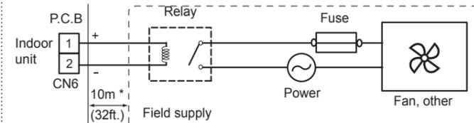
\*:Make the distance from the PC board to the Relay Unit within 10 m (32 ft.).
