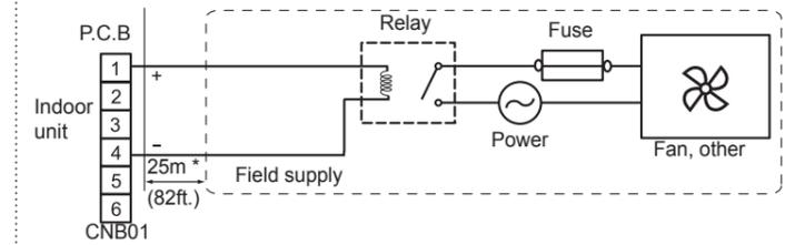
\*:Make the distance from the PC board to the Relay Unit within 25 m (82 ft.).
