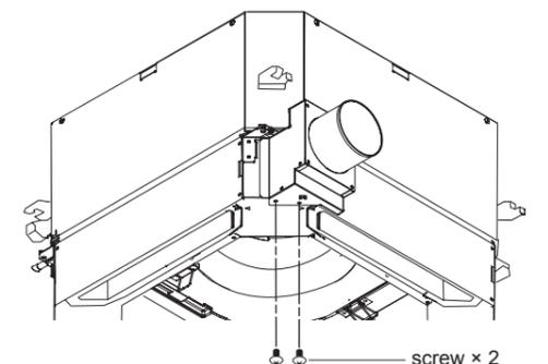
\* When using the "UTZ-KXGC" kit for high humidity, please first cut off and remove the heat insulation as shown in the figure.
