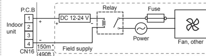
\*:Make the distance from the PC board to the Relay Unit within 150 m (492 ft.).
