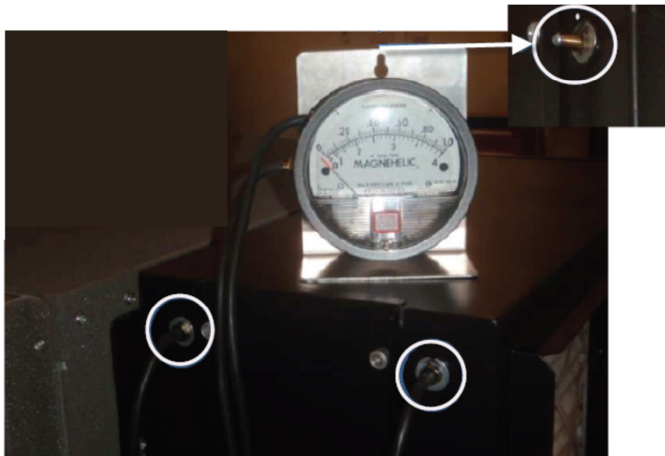
Figure 6: To utilize meter connections, remove the screws from the connection port and install the meter hose.
