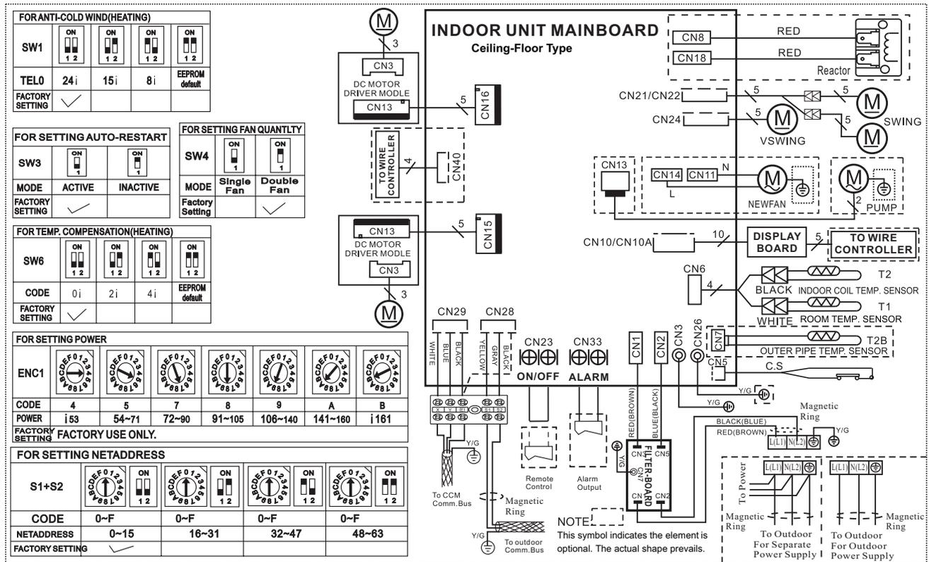
Fig. 16 — Wiring Diagram - Size 58K
