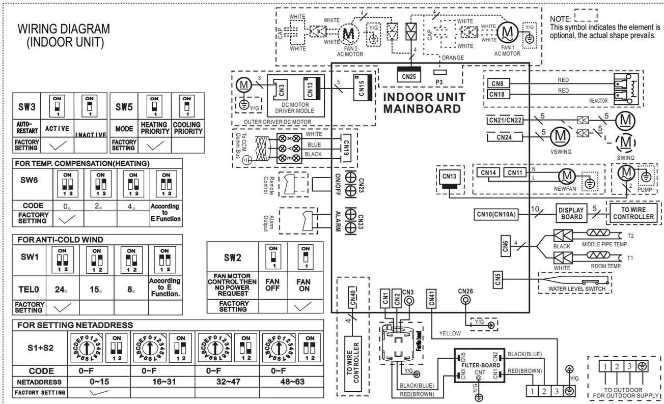
Fig. 13 — Wiring Diagram - Sizes 18K and 24K
