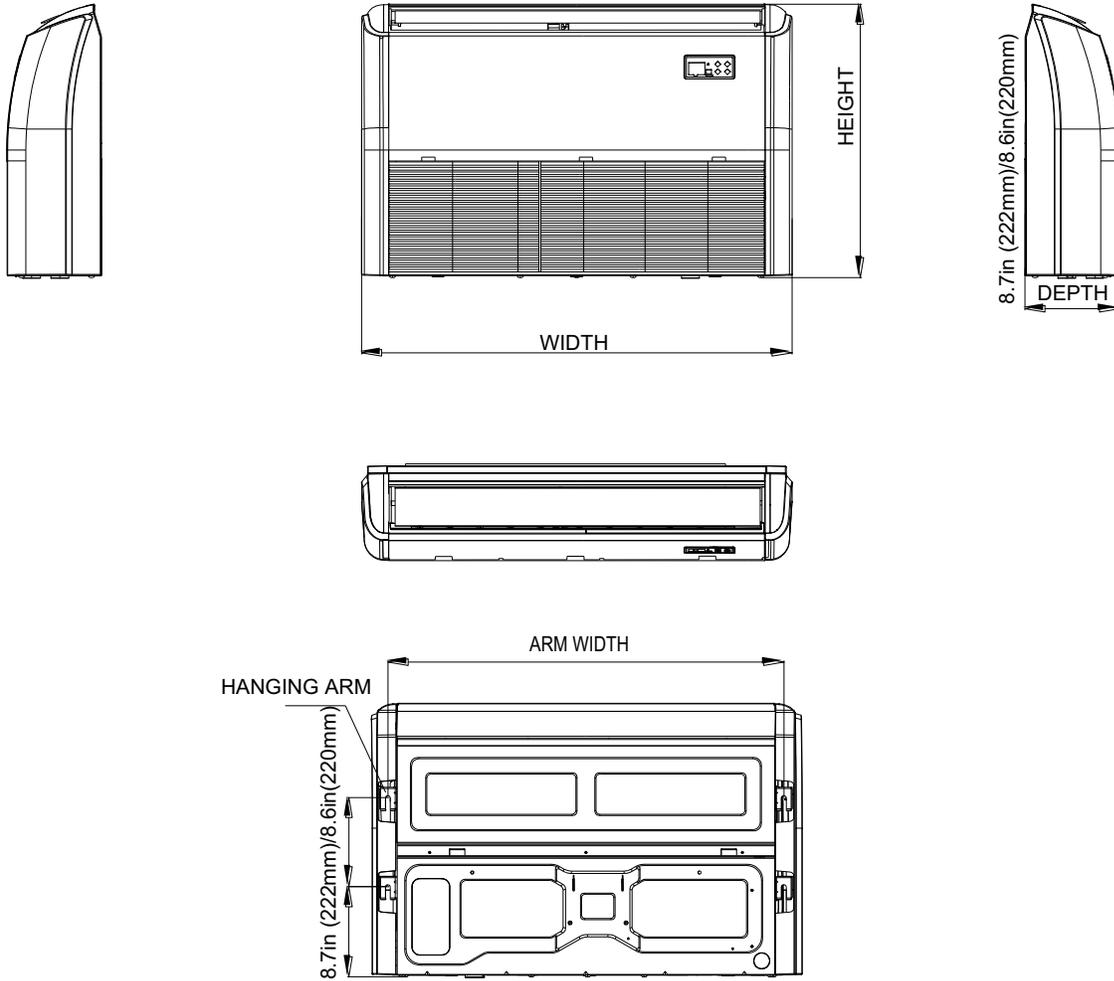
**Fig. 5 — Indoor Unit Sizes 18K-58K**
