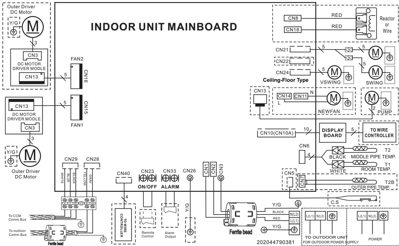
Fig. 15 — Wiring Diagram - Size 48K
