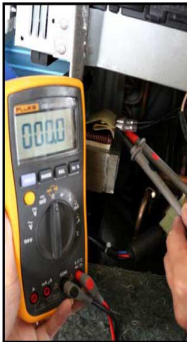
Fig. 18 —Test the Reactor Resistance
