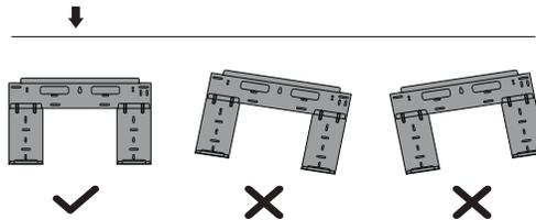
Fig. 9 — Mounting Plate Orientation
