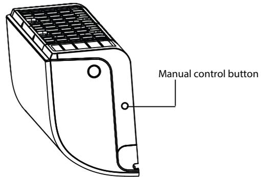
**Fig. 36 — Test Operation**
