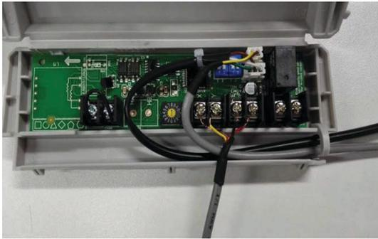
**Fig. 32 — Connect the cable to the board**
