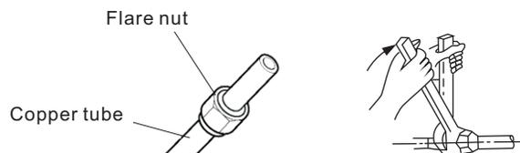
**Fig. 26 — Tighten the flare nut**
