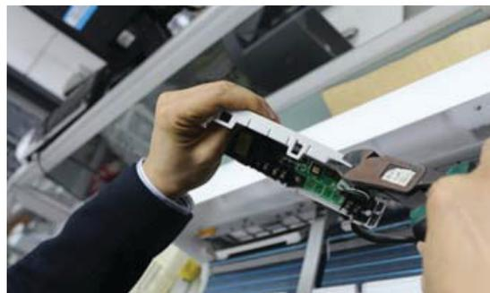
Fig. 30 — Cut a hole on the multi-function board
