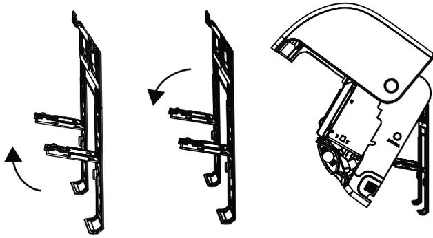
**Fig. 16 — Use Holder to Prop up the unit**
