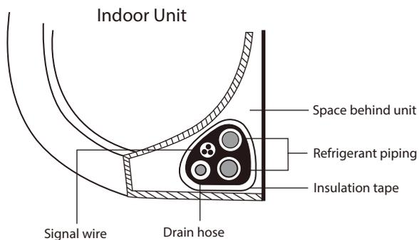
Fig. 28 — Bundle drain hose, refrigerant pipes, & signal cable
