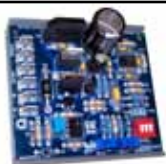
FIGURE 20B - Signal Conditioner in Option AG21
