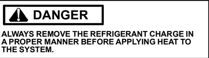
These models use the FasTest Access Fitting System, with a saddle that is either soldered to the suction and liquid lines or is fastened with a locking nut to the access fitting box (core) and then screwed into the saddle. **Do not remove the core from the saddle until the refrigerant charge has been removed. Failure to do so could result in property damage or personal injury.**
