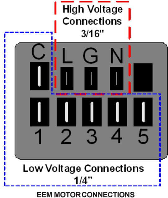
1. Using a voltmeter, check for 230 volts to the motor connections L and N. If 230 volts is present, proceed to step 2. If 230 volts is not present, check the line voltage circuit to the motor.
