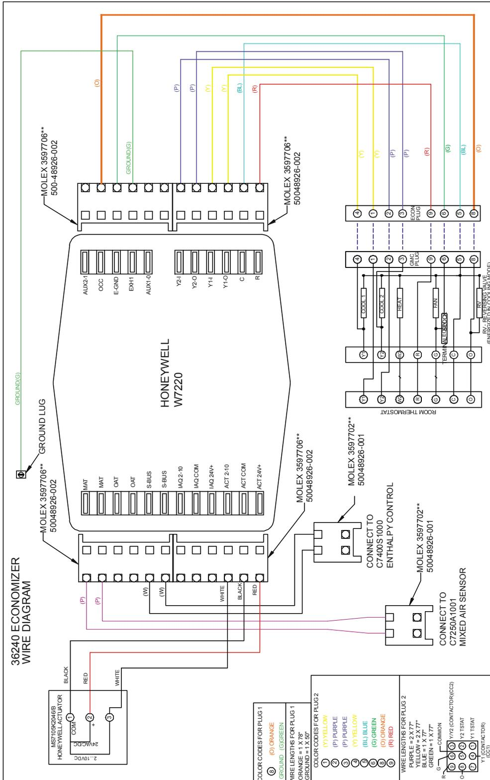
Wiring is subject to change. Always refer to the wiring diagram on the unit for the most up-to-date wiring.
