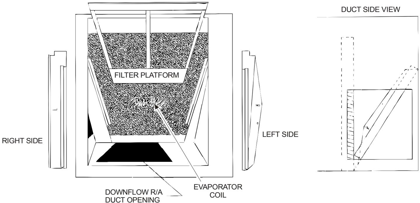
Filter Size: 14" x 25" x 2" (Requires 2 filters) - Measurement in inches
