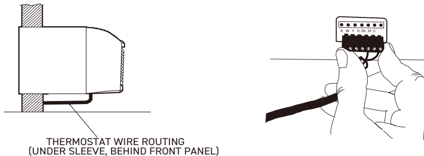
Figure 401(Wiring Thermostat To Unit)
