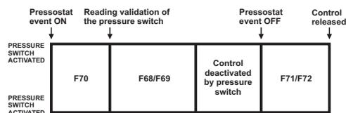
**NOTE 1:** For safety reasons, if controller registers 3 high pressure or 3 low pressure events in one hour period, three outputs of controller will be turned OFF: Compressor, Defrost & Fan display on controller will show alarm message  - High pressure alarm or  - Low pressure alarm. To reset  and  alarms a manual intervention is required. To manually reset: short press  key on controller to navigate  option, short press  key, select the option ON and press  key.
